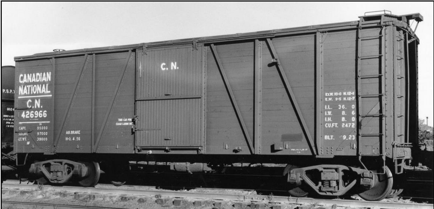
CN car with six foot door. The cars was built in 1923, and by the time of this 1957 photo had been modernized with an outside metal roof, cast steel trucks, and AB brakes.
