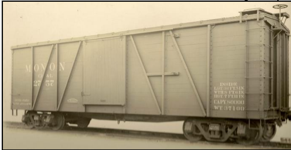
As-built Monon Fowler. Pullman builder's photo.
