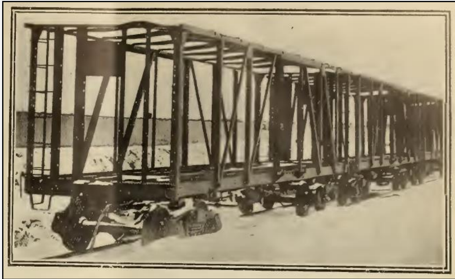
Some of the first Dominion-built cars head from Dominion's plant to the CP's Angus Shops to be sheathed and painted. Photo from Railway and Marine World magazine, January 1910.
