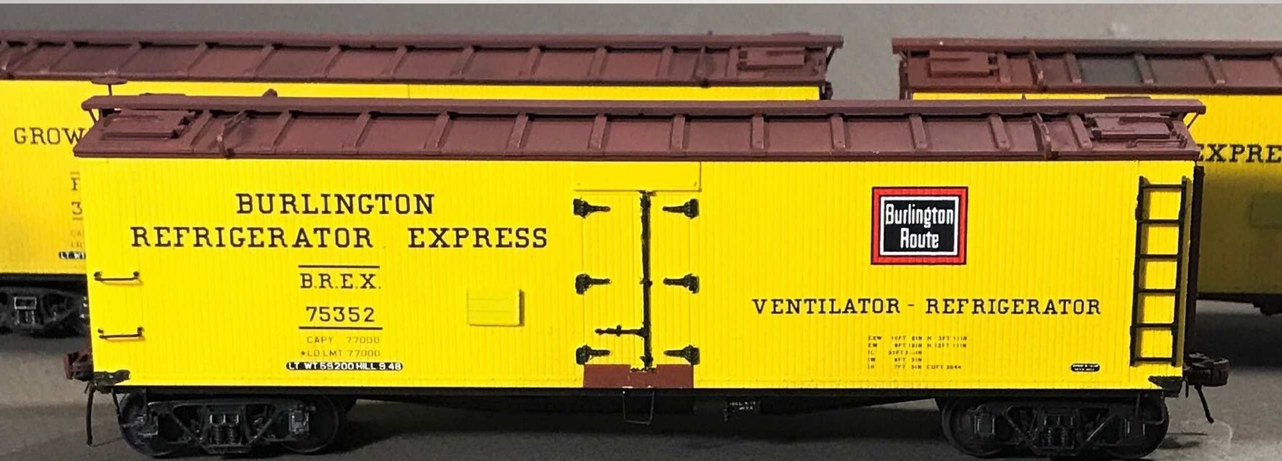
Note this is the rebuilt version with the FGEX Hutchins roof for a backdated model see Bill Welch article in Prototype Railroad Modeling, Vol. I, Speedwitch Publications “The Burlington Refrigerator Express Company’s Signature Wood Sheathed Reefers”
